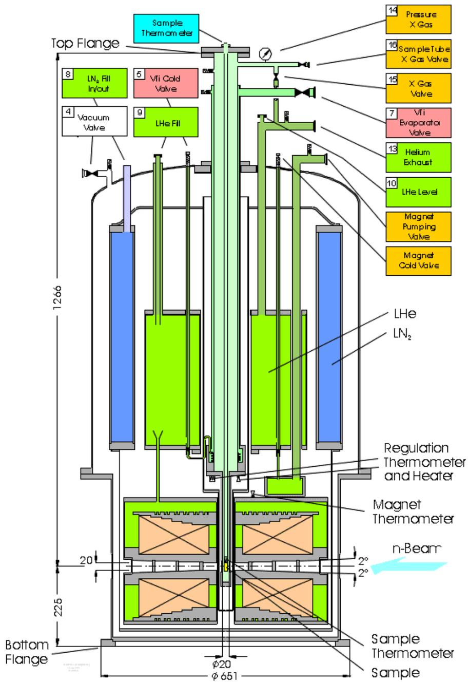
**Fig. 17:** Cross section through a typical high-field magnet system (see text).
