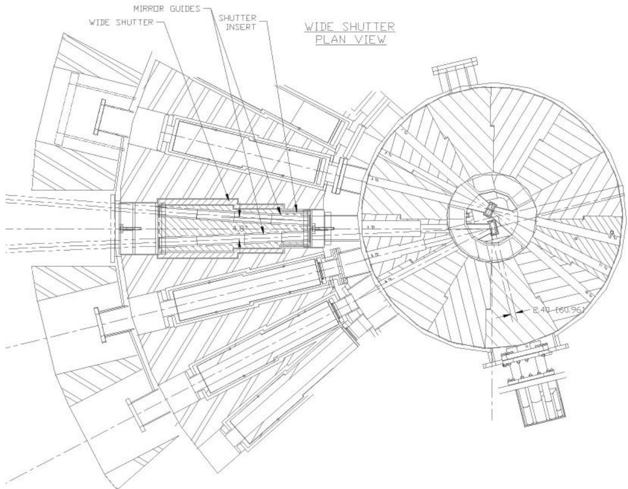
**Fig. 8:** Moderator / wide shutter configuration on the SNS reflectometry beamline.
