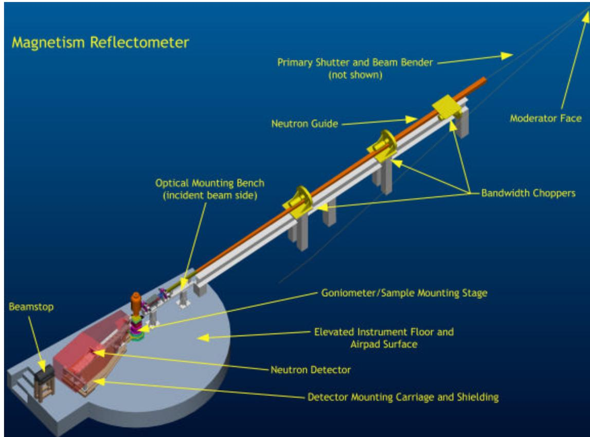
**Fig. 3:** The Magnetism Reflectometer consists of the following components: channel beam bender (not shown), tapered neutron guide, bandwidth choppers (yellow), polarizing optics, sample area (with a cryostat mounted), detector assembly (analyzing optics, detector, shielding) and a beam stop.
