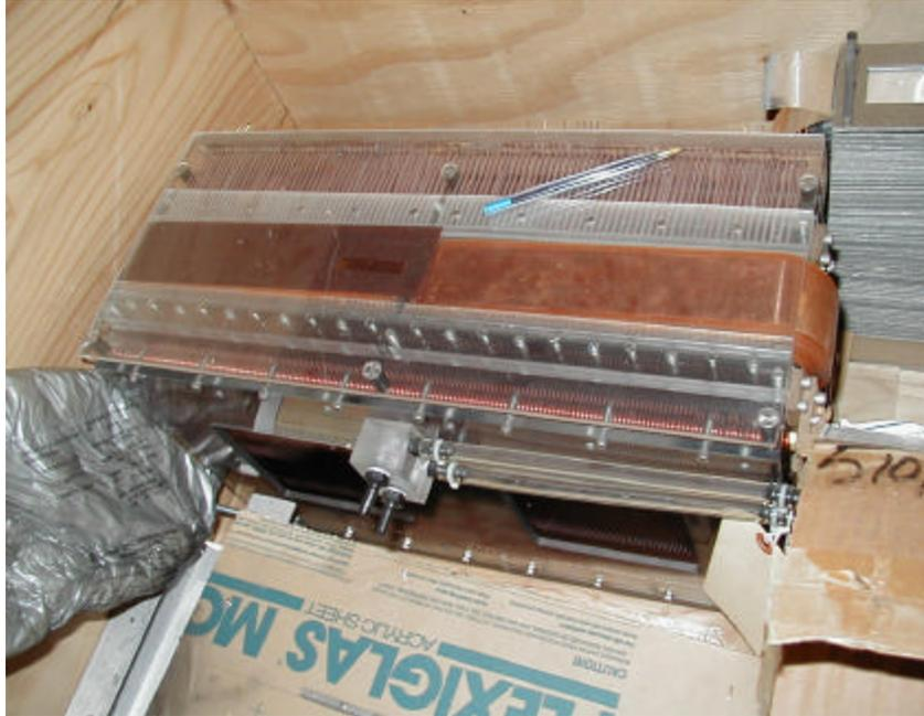
**Fig. 15:** Prototype of the Drabkin energy filter developed by C. Majkrzak and L. Passell.
