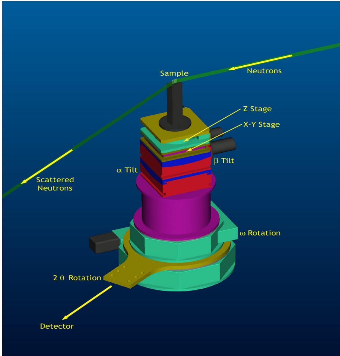
**Fig. 16:** Required angular and linear movements of the goniometer.
