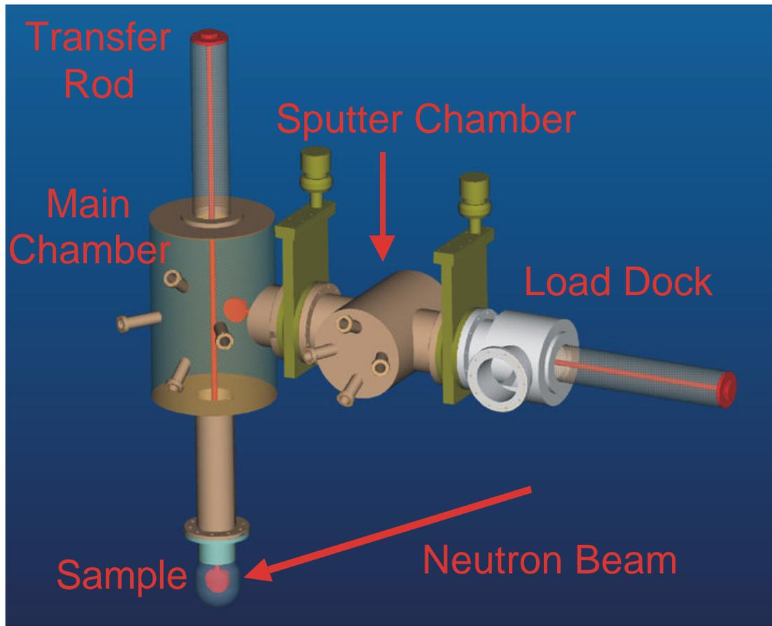
**Fig. 20:** Schematic layout of the UHV system.
