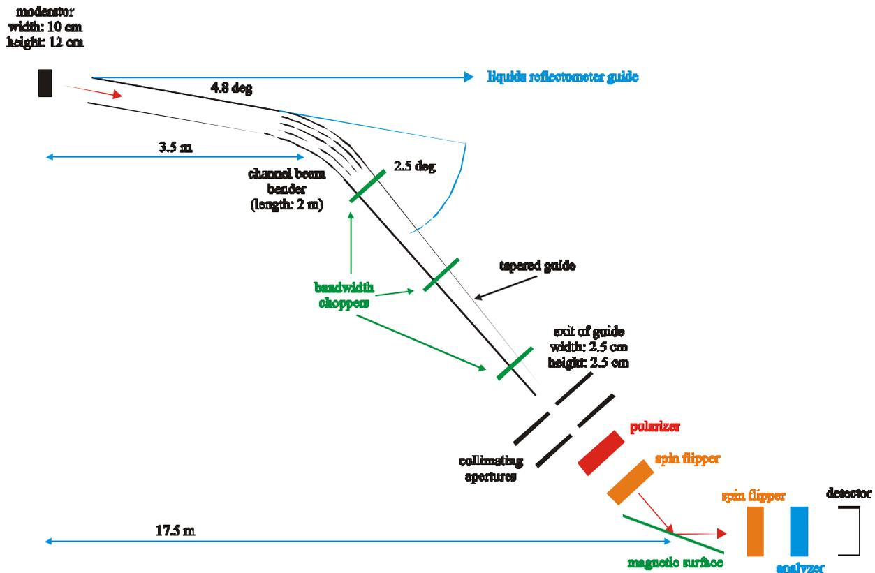
**Fig. 2:** Neutron beam optics of the magnetism reflectometer (top view, schematic).
