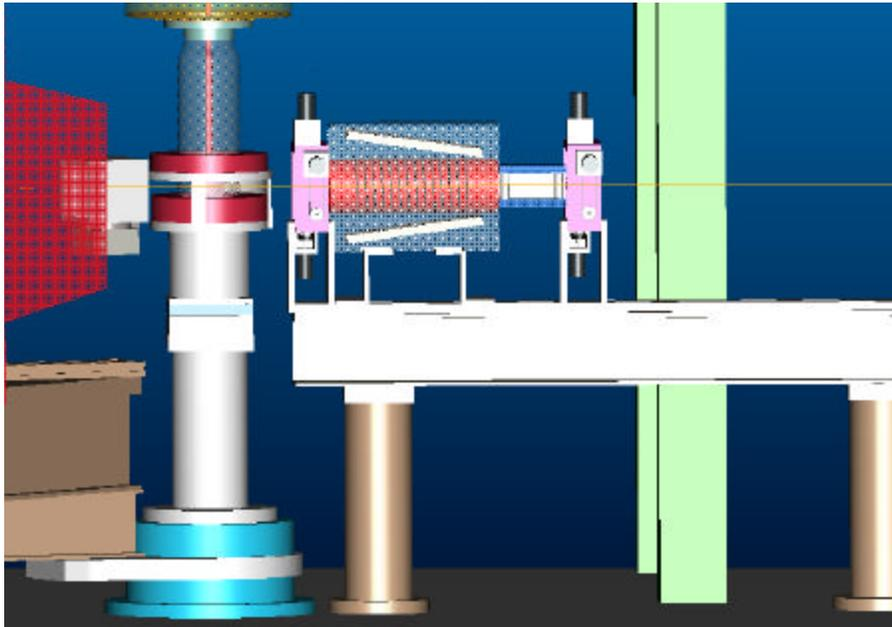
**Fig. 13:** Incident beam polarizing optics (spin flipper and polarizer mounted between aperture systems).
