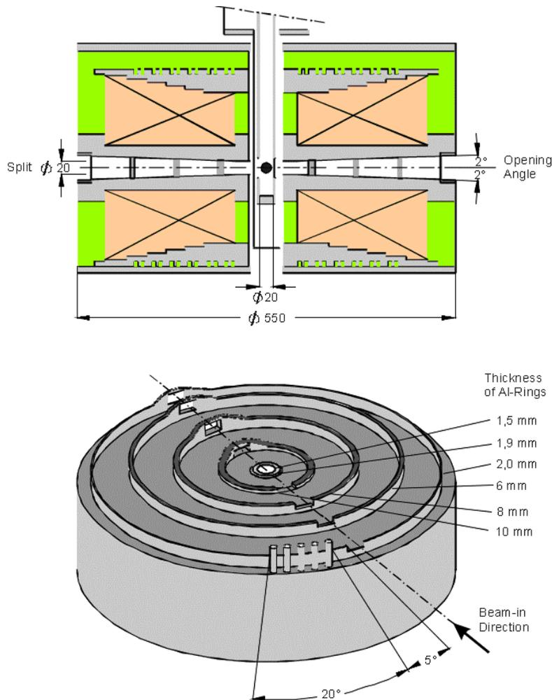
**Fig. 18:** Spacer ring arrangement of a typical high-field magnet system (see text).
