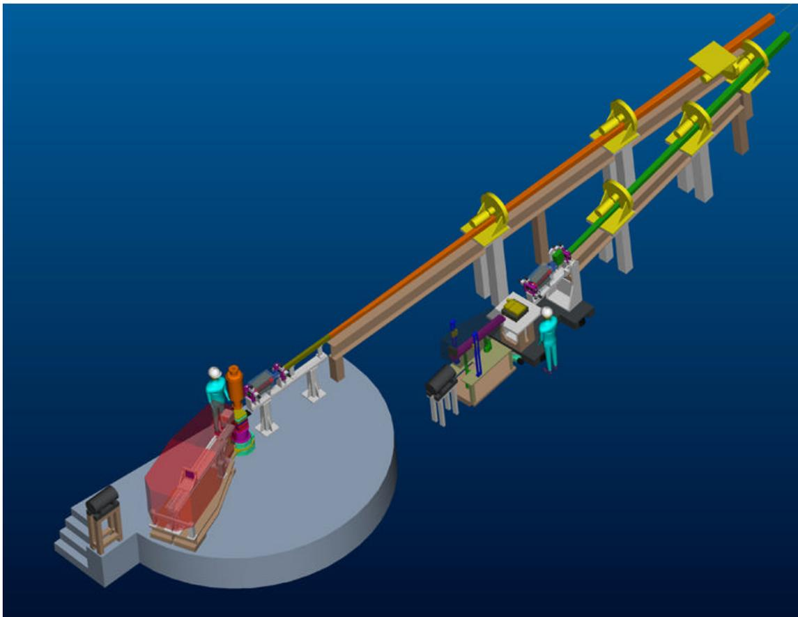
**Fig. 1:** The SNS reflectometry beamlines: The upper beamline represents the Magnetism Reflectometer, the lower the Liquids Reflectometer.
