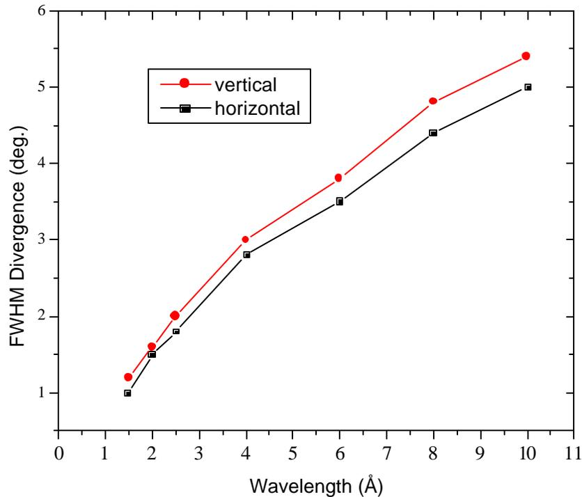
**Fig. 10:** Wavelength-dependence of the beam divergence at the exit of the tapered guide.
