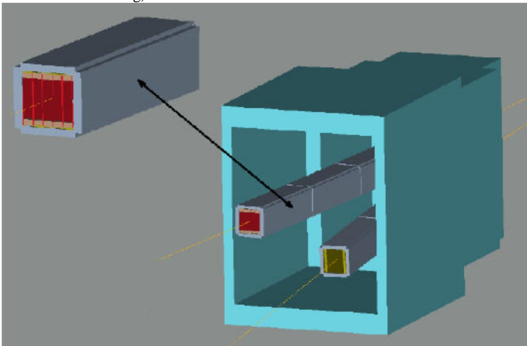
**Fig. 9:** Schematic representation of the channel beam benders integrated into the main beamline shutter. One of the four straight bender sections is depicted enlarged.
