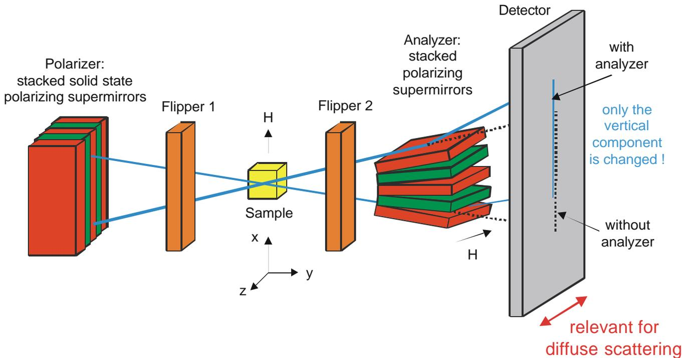
**Fig. 11:** Spin-handling system of the Magnetism Reflectometer.
