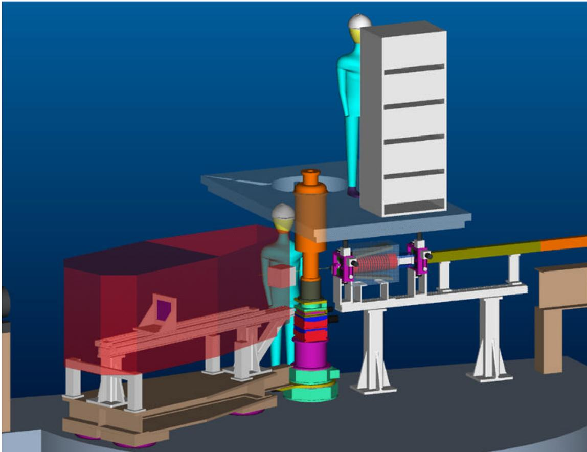
**Fig. 4:** Detailed view of the beamline close to the sample position. If a cryostat is in use, sample loading will be done from a platform atop the sample area. Otherwise sample access is possible from the instrument floor
