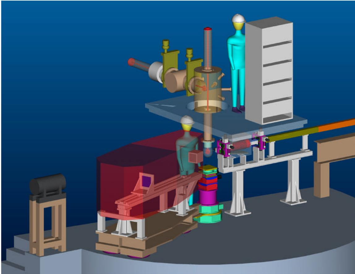
**Fig. 19:** UHV system for in-situ polarized reflectometry experiments on ultrathin magnetic films (for clarity reasons the sample magnet is suppressed).
