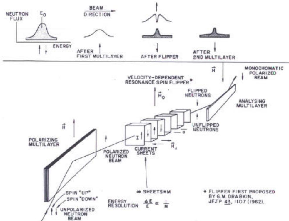
Fig. 14: Basic principle of the Drabkin energy filter.
