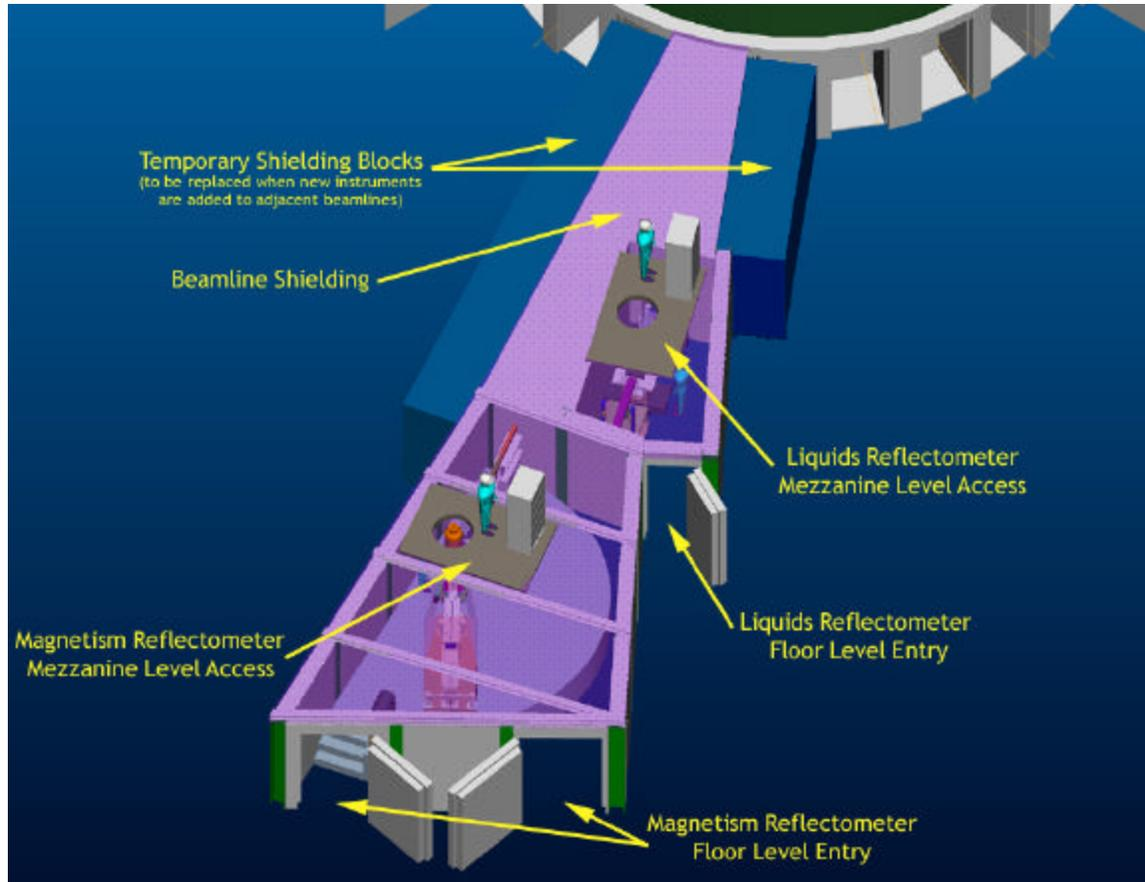
**Fig. 21:** Preliminary arrangement of shielding and instrument enclosures at the reflectometry beamlines. The shielding blocks that constitute the roof are suppressed for clarity reasons.
