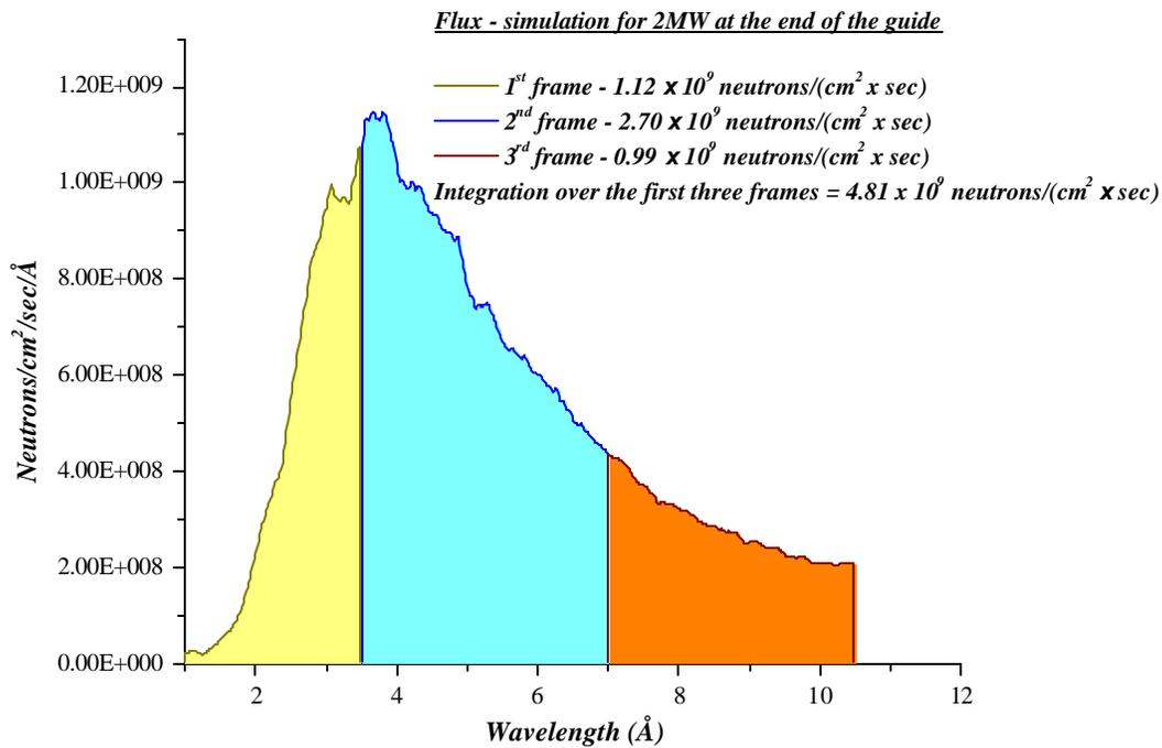
**Fig. 6:** Calculated neutron flux at the exit of the tapered neutron guide of the SNS Magnetism Reflectometer. Note that the flux is pulsed with a frequency of 60 Hz and has an intrinsic time/wavelength resolution of 0.4% (see also section 2.1).
