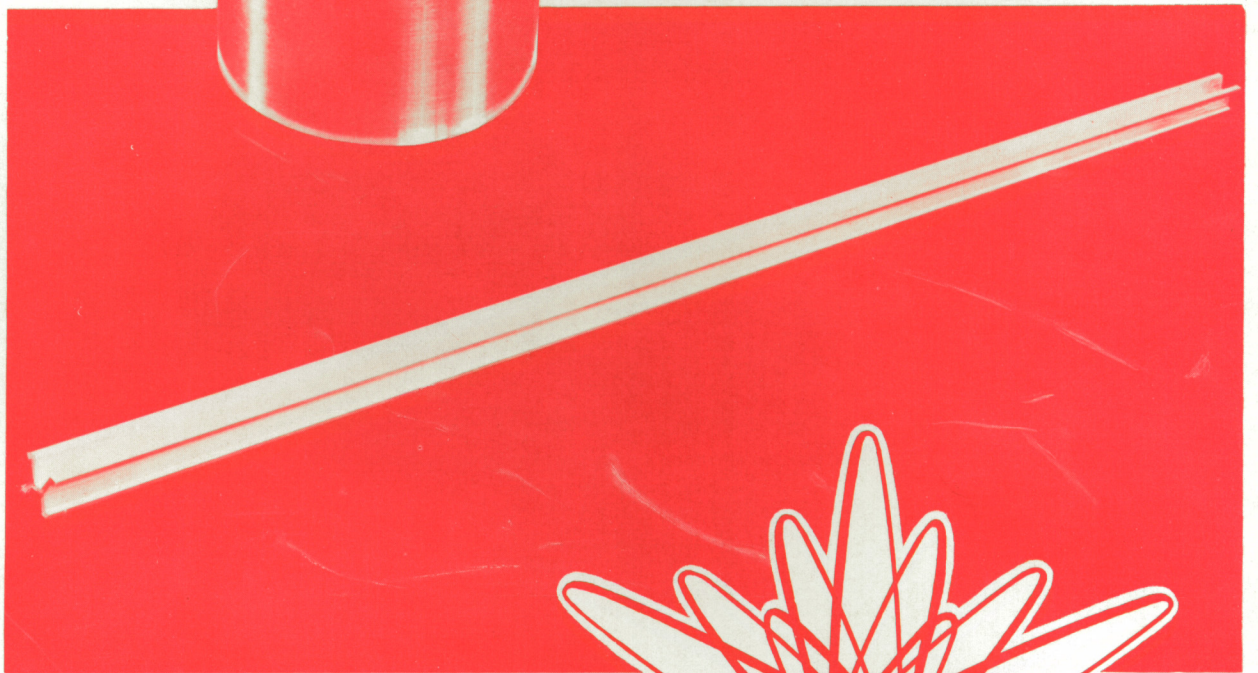
U.S. Prototype Meter Bar 27, the standard of length of the United States from 1893 to 1960. On October 14, 1960, the meter was redefined in terms of a wavelength of the krypton 86 atom.
