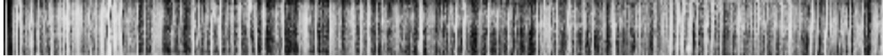
Figure 5.5. A linescan image of NGRIP ice core interval 2528.35–2530.0 m depth. Gray layers, annual cloudy bands; annual layers are about 1.5 cm thick. Age of this interval is about 72 ka, which corresponds with Greenland Interstadial 19. (Svensson et al., 2005)
