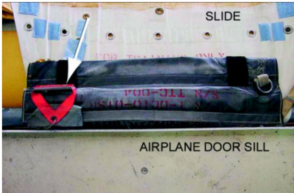
Figure 3. FedEx's MD-11/-10 emergency evacuation door trainer, with the girt flap assembly in place, as it would appear when the door/slide is opened. The arrow indicates the manual inflation handle.
