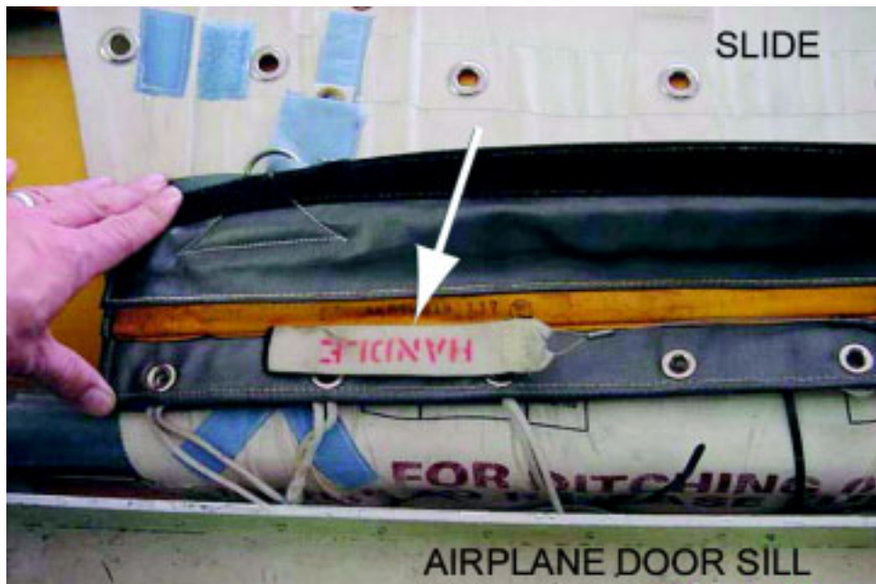
Figure 4. FedEx's MD-11/-10 emergency evacuation door trainer, with the girt flap assembly lifted. The arrow indicates the slide/raft disengage handle.
