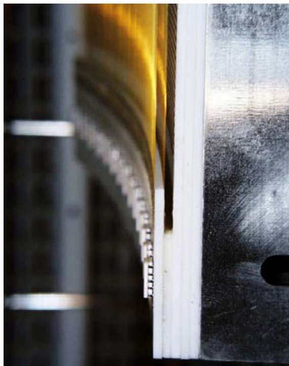
Fig. 2.19. Edge view of curved, wire segment. Curvature eliminates parallax error (in horizontal plane in this example); position readout yields electronic accuracy better than 1 mm.
