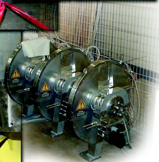
Clockwise from top left: evacuated scattering chamber for the backscattering spectrometer (installed in final position on the instrument); schematic of VULCAN; (middle images) poured-in-place base beam-line shielding for the backscattering spectrometer (viewed from opposite ends); bandwidth-selection choppers for the backscattering spectrometer being tested in the lab; and installation of the guide sections in the shutter insert for the backscattering spectrometer.
