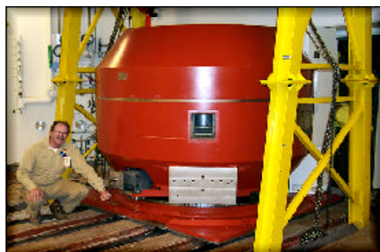
New monochromator shield and rail-support system at HB-1.
