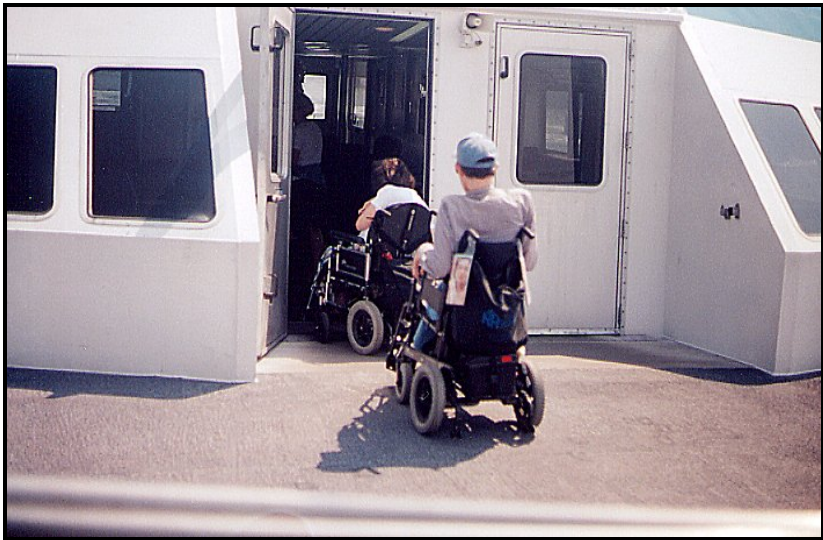
Figure 3-2 Access Through the Passenger Cabin Bow Doors
