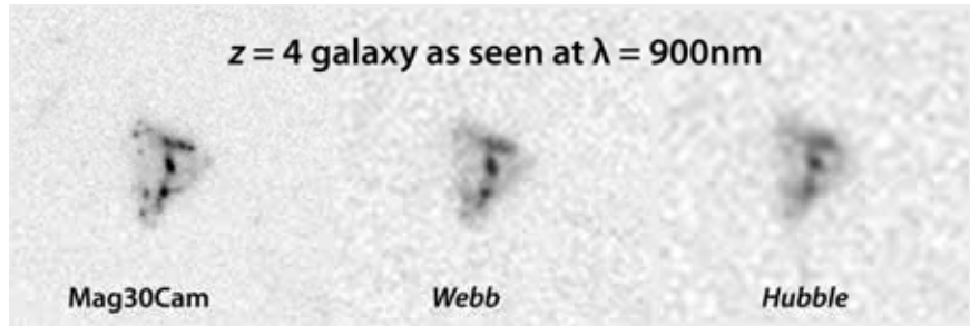
Figure 4.1-30. The Improved Resolution and Sensitivity of TPF-C's WFC Compared with Webb and Hubble. The Simulated Object is an L^* galaxy at z = 4 Observed in a Broadband Filter Centered at \sim 900\text{ nm} .
