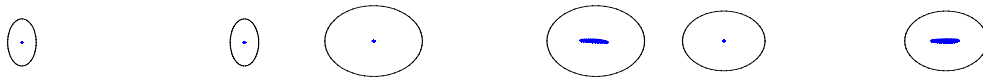
Figure 3.3-40. Spot diagrams at three positions inside the system. (a) telescope focus, (b) occulting mask, (c) final focus. The ellipse/circle represents the Airy disk size at the corresponding location. In each case, the middle of the field (left) and the worst-case 2 arcsec field (right) are shown.
