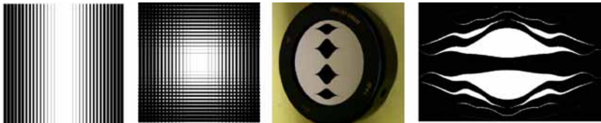
Figure 5.3-3 Bar Code Masks and Shaped Elliptical Masks. From left to right: 1-D bar code mask; 2-D bar code mask; four-aperture mask elliptical mask; multi-aperture elliptical mask.
