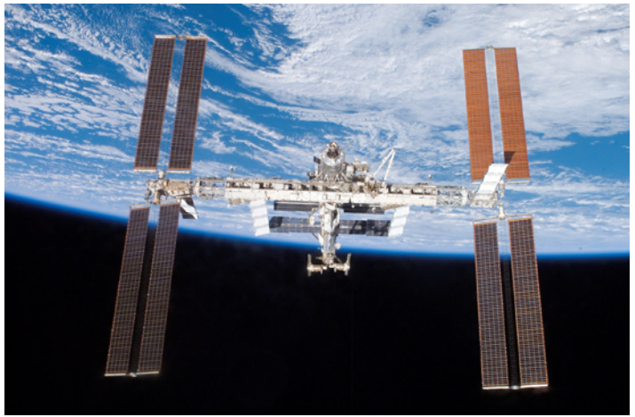
The entire array of expansive solar panels is visible at the edges of the above image taken by the Shuttle Atlantis Crew after leaving the ISS to return to Earth. Also visible above are many different types of modules, a robotic arm, another impressive set of solar panels, and a supply ship. Construction began on the ISS in 1998. (NASA)
