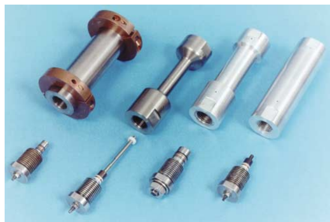
Fig. 9. A selection of Ti–Zr alloy and Al. alloy ISIS High Pressure Intensifier cells with Bridgman seals.
