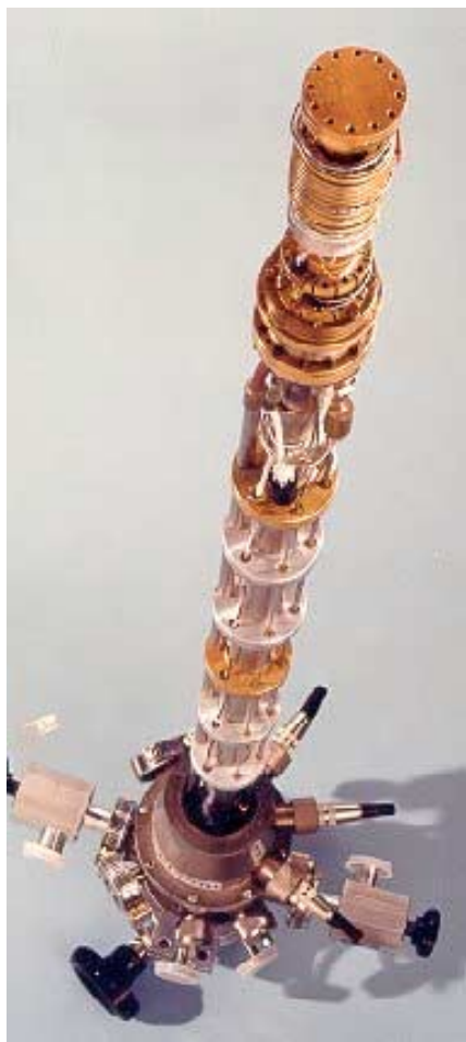
Fig. 3. “Charlie” Dilution Fridge Insert for 50 mm Orange Cryostats.
