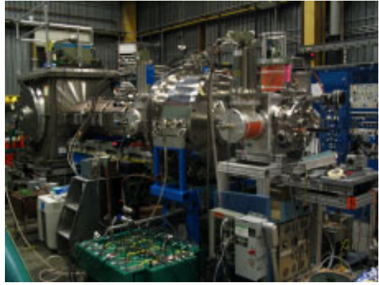
The Neutralized Drift Compression Experiment at the LBNL to study the limits of compression of ion beams in the presence of a neutralizing plasma. Large compression of the ion beam is required for using the ion beams to perform experiments to investigate Warm Dense Matter.
