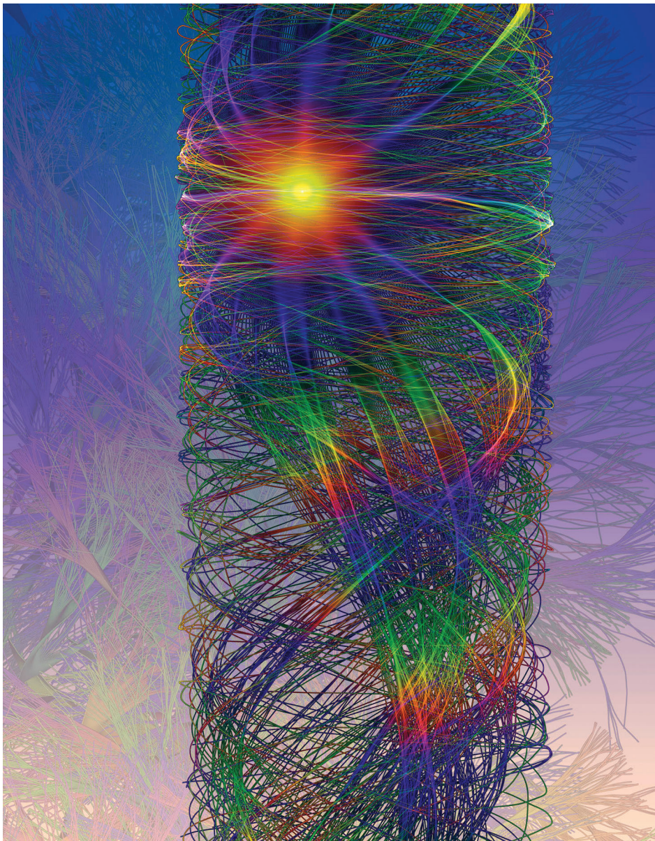
Figure 3b. Theoretical simulations of electron flow in nanostructures: Flow of electrons injected at the “bright spot” into a 500 nm diameter “nanowire.” Electrons are scattered due to interactions at the wire surface. Variation in the quantum phase of the scattered electron waves is indicated by changes in color. The dynamics of such electron scattering affects the electronic properties of the wire, its resistance, the speed of response to external stimuli, and coherence of information flow along its length (courtesy E.J. Heller, Harvard University).
