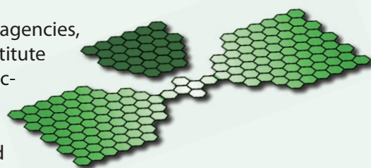
Concept of a switch made from a graphene sheet. Here a molecular quantum dot (center, white) is connected to graphene electrodes through narrow constrictions. A coplanar graphene side gate (dark green) controls charge flow through the switch. Reproduced by permission from Physics Today , © 2007 American Institute of Physics.
