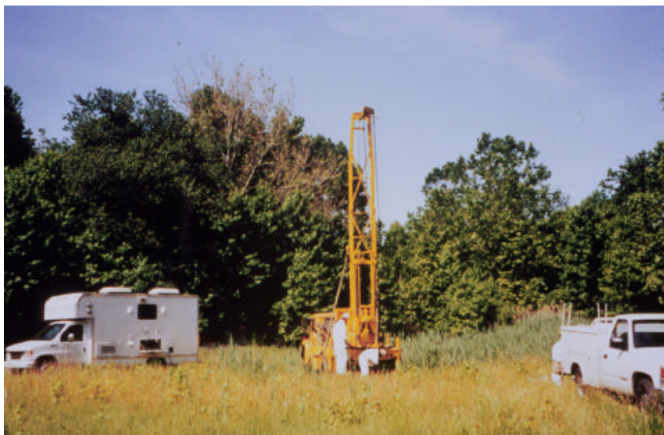
A Real Time Analytical Platform (RTAP) contained in the truck on the left is being used to monitor chemical warfare agents during intrusive sampling.
