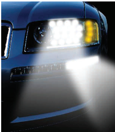
Solid-state headlights using light-emitting diodes (in development) could improve vehicle efficiency. (Courtesy of Visteon Corporation)
