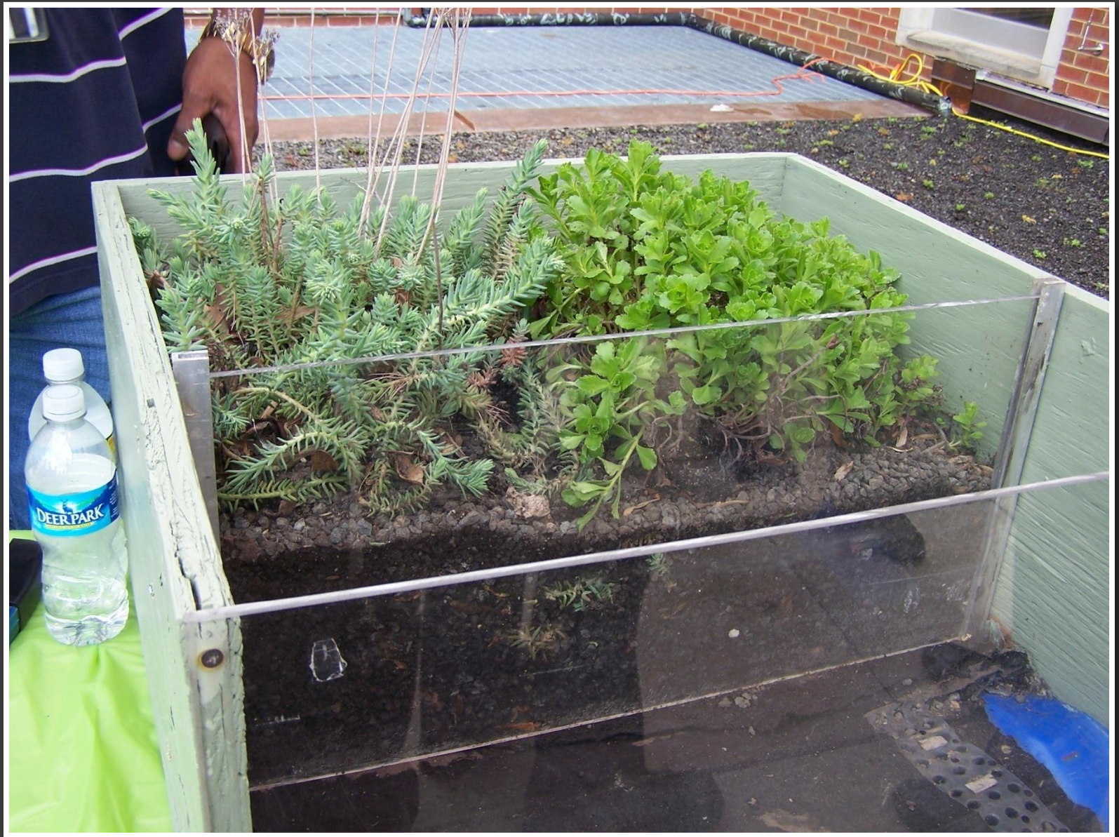
A sample of the roof layers and plant materials was also on display.
