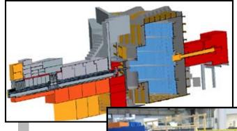
ror guide in the incident flight path boosts the performance at the lower end of this range. The sample and detector vacuum chambers provide a window-free final flight path and incorporate a large gate valve to allow rapid sample changeout. A new  $T_0$  neutron chopper will not only
