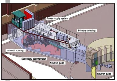
the estimated time-averaged sample flux of  $10^7$  n/cm<sup>2</sup>s around  $\lambda = 1$  nm. This yields the highest available data accumulation rate. In addition, the wavelength distribution width at any time is well below 0.5%, causing the resolution in momentum transfer to increase significantly compared with reactor instruments with 10% or more wavelength distribution width.
