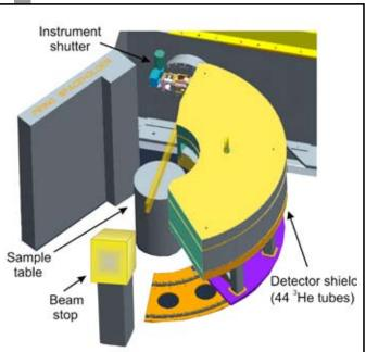
1.54 Å, and (117) 1.12 Å. The takeoff angle from the monochromator is fixed at 90°, and the minimum peak full width at half maximum (FWHM) is 0.2°. There are two choices of premonochromator collimation ( $\alpha_1$  = 12' or open) and three choices of presample collimation ( $\alpha_2$  = 16', 21', or 31') that allow the operation of the instrument in high-resolution or high-intensity modes.
