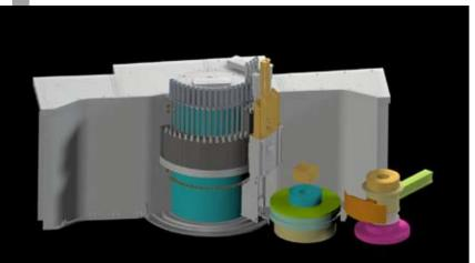
of strong magnetic fields at the sample position and to simplify future polarization analysis, the amount of ferromagnetic material has been minimized in the construction of this instrument.
