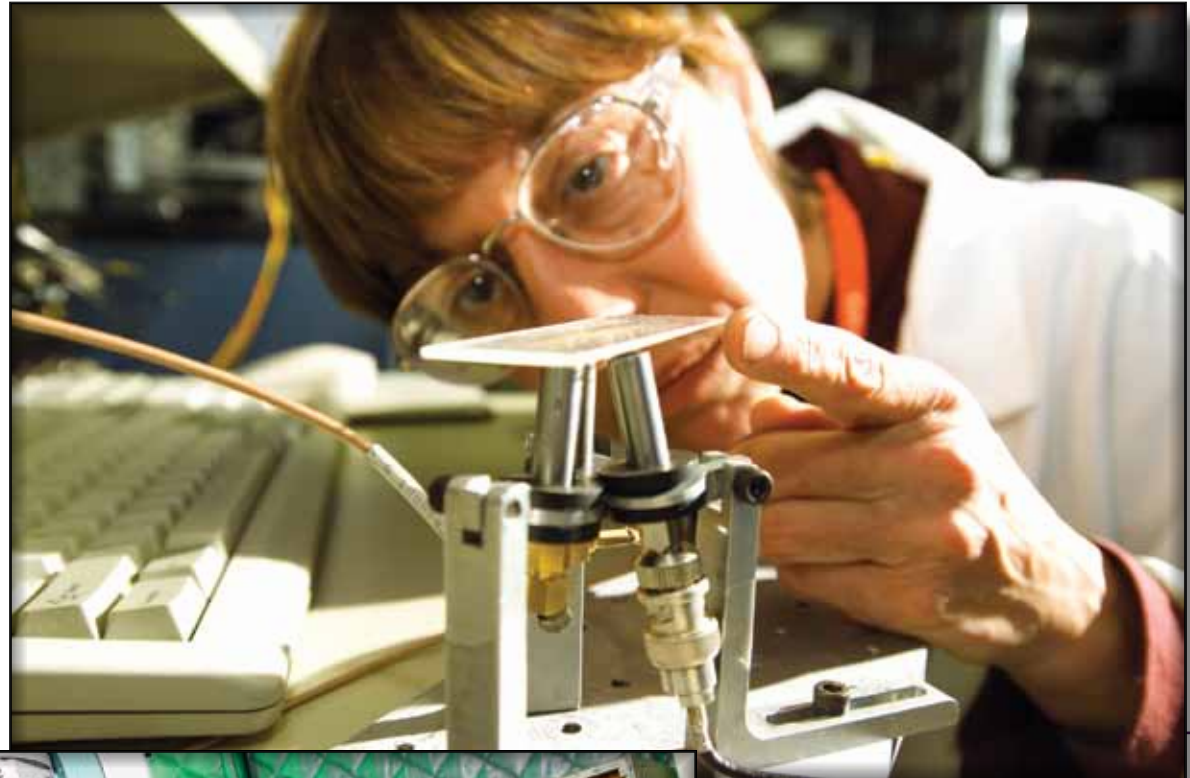
Laura Riester adjusts a specimen for measuring elastic properties using resonant ultrasound at HTML.
