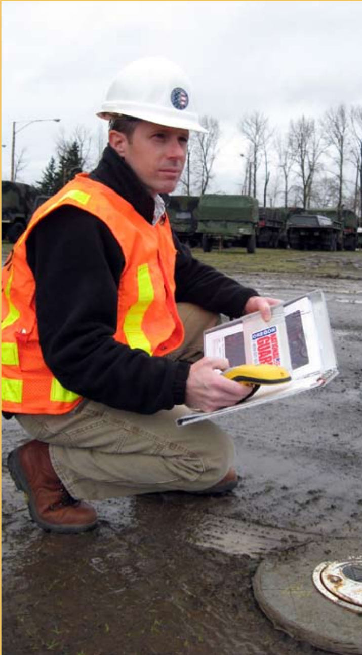
Jim Arnold collects location coordinates of a groundwater monitoring well with a handheld Global Positioning System (GPS) unit at one of his project sites.
