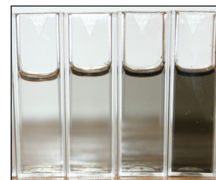
Figure 2: Multi-walled nanotubes stabilized in natural organic matter
