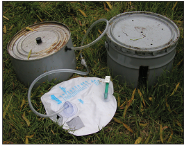
Figure 5. Seepage meters. A. Large seepage meter with attached housing unit. B. Small seepage meter with housing unit.
