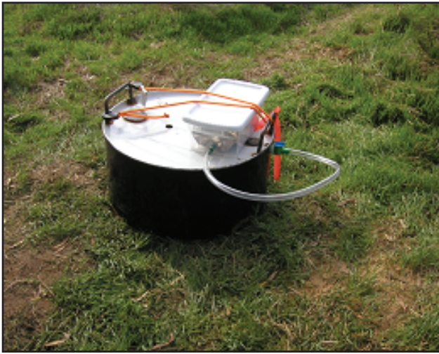
Figure 5. Seepage meters. A. Large seepage meter with attached housing unit. B. Small seepage meter with housing unit.
