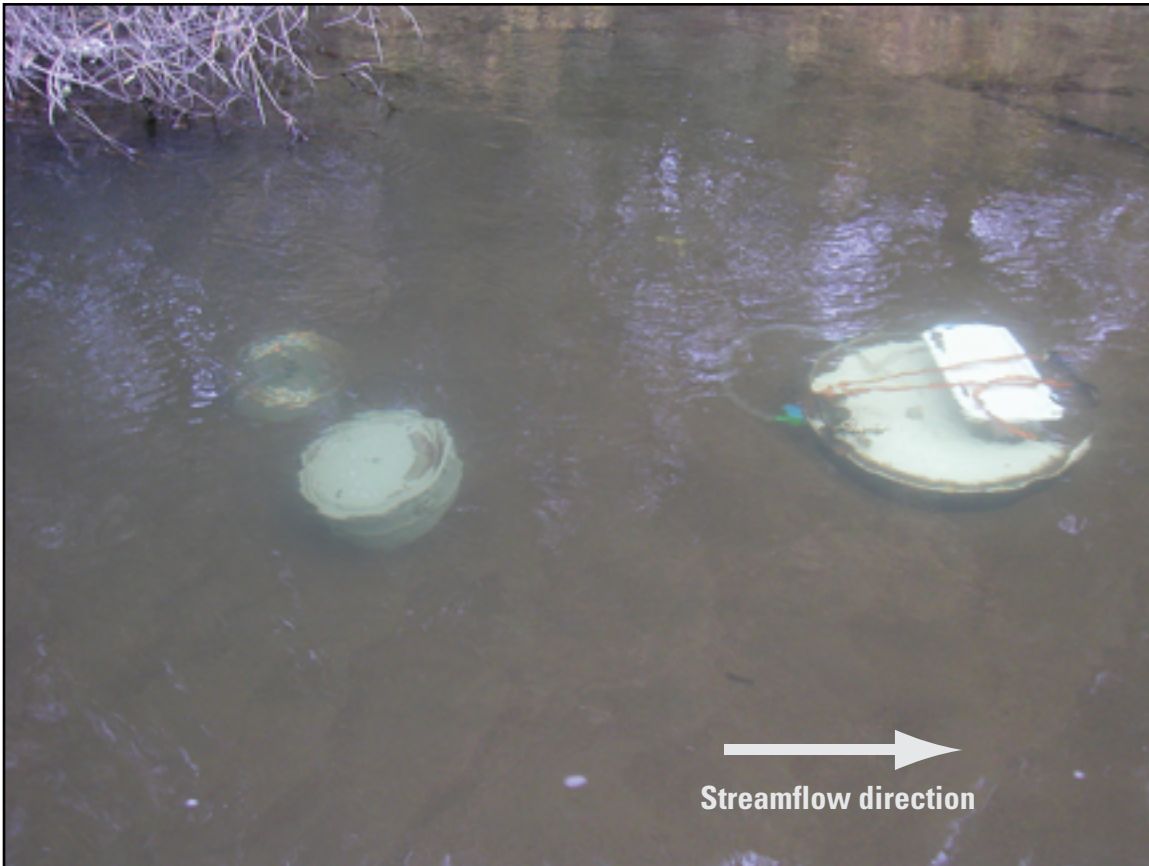
Figure 6. Field deployment of paired seepage meters.
