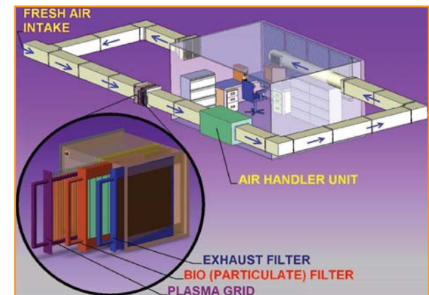
Diagram of AGT's Enhanced Plasma System for Indoor Air Quality, which destroys all types of captured microorganisms while reducing concentrations of airborne VOCs.
