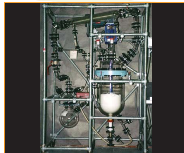
Pictured above is the device used to synthesize TDA's nanoparticle-anchored plasticizers, which soften polyvinyl chloride (PVC), keep plastics soft longer, and do not escape.
