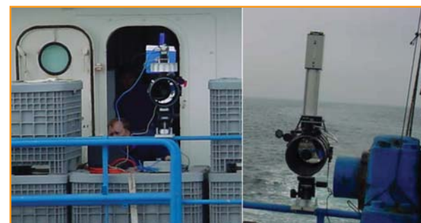
duoThane ® transmitter and receiver mounted on an oil spill clean-up vessel demonstrating the effectiveness of detection of leaks from pipelines that run under waterways.
