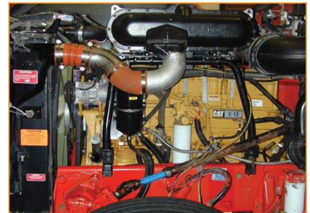
Membranes within the black housing mounted over the diesel engine pictured above generate NEA from cooled turbocharged air.
