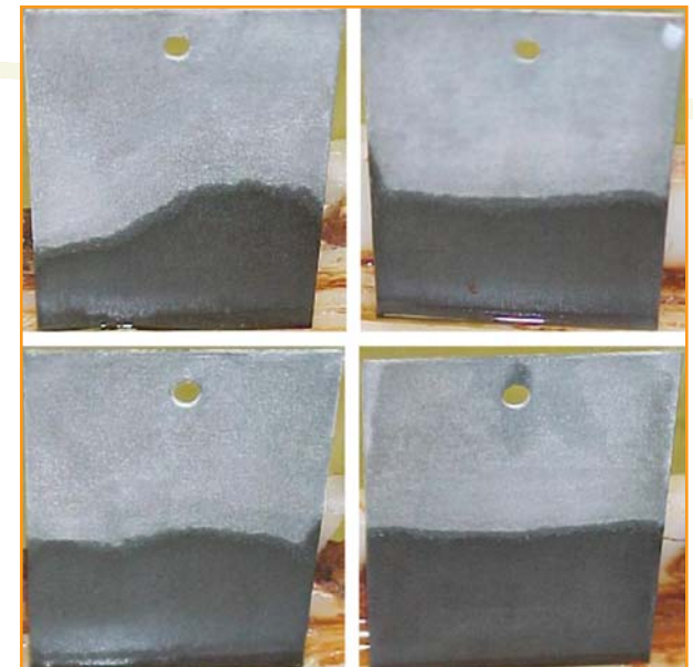
Aluminum 2024-T3 panels prepared with Lynntech conversion coating. No pitting is observed after 336 hours of salt fog spray testing.
