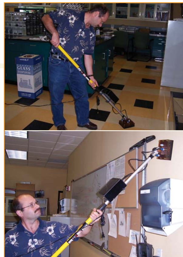
Demonstration of the plasma cleaner to treat horizontal and vertical surfaces.
