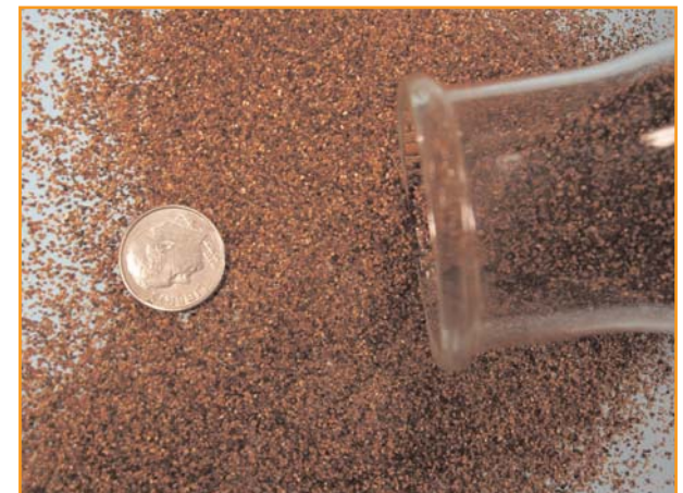
ADA developed and commercialized an arsenic removal POU/POE drinking water system using Amended Silicate™ sorbents (pictured above with a dime to indicate scale).
