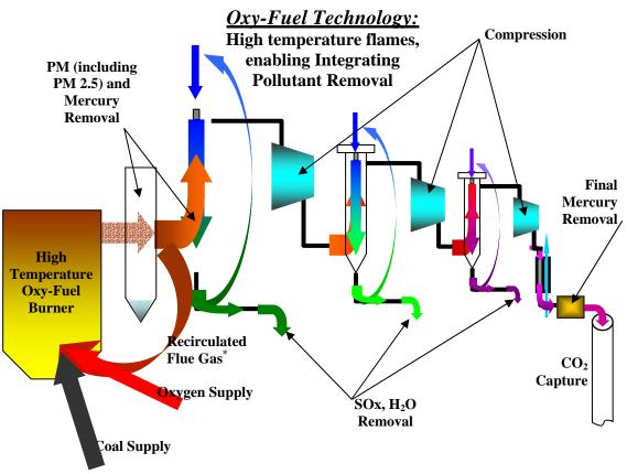
\*In retrofit applications, recirculated flue gas is used to balance heat transfer to convective zones
