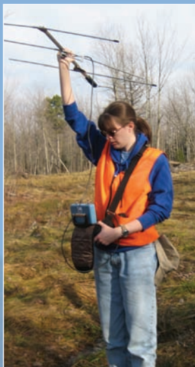
Megan locates individual birds within the habitats she is studying via radiotelemetry. Here, she uses a receiver with antenna to pick up a radio signal from a small transmitter placed on a bird.
