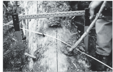
Figure 3—When the line-intersect method is used, diameters of qualifying logs are measured where the transect line intersects the central axis of the log.
