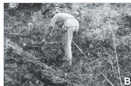
Figure 2—Calipers function as a square when using strip-plot method (A). Two lengths of the calipers denote the outer boundaries of the plot and the place to where the length is measured and the large (or small) diameter is taken (B).
