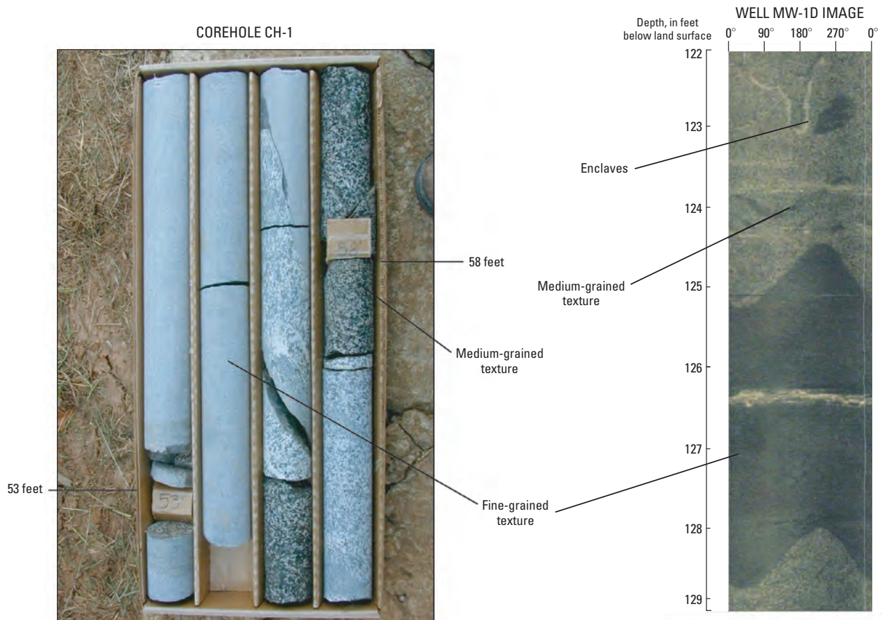
Figure 11. Whole rock core from corehole CH-1 (location in fig. 5) and optical televiewer image of well MW-1D showing examples of alternating fine- and medium-grained texture in the quartz diorite bedrock at the Langtree Peninsula research station, North Carolina.
