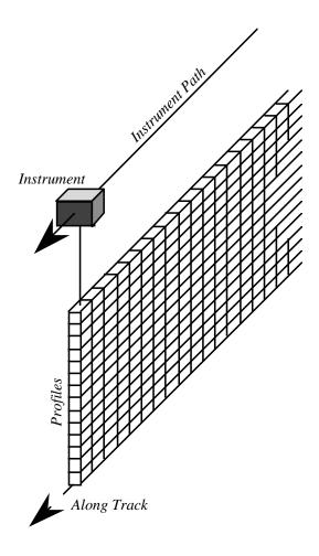
Figure 5-2. A Swath Derived from a Profiling Instrument
