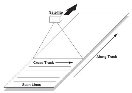
Figure 5-1. A Typical Satellite Swath: Scanning Instrument
