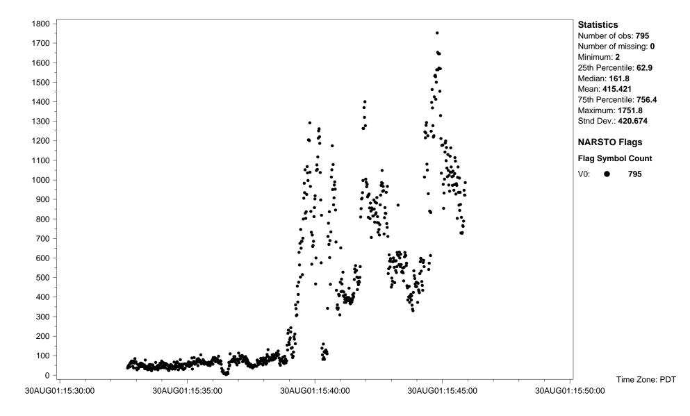
Site ID: **PC01CABCCONV** Variable name: **Particles: count** Units: **number/cm3** Basis: **channel 1** Sampling interval: **1 second** Sampling frequency: **Same as sampling interval** Observation type: **Particles** Particle diameter--lower bound (UM): **0.130** Particle diameter--median (UM): **0.140**
