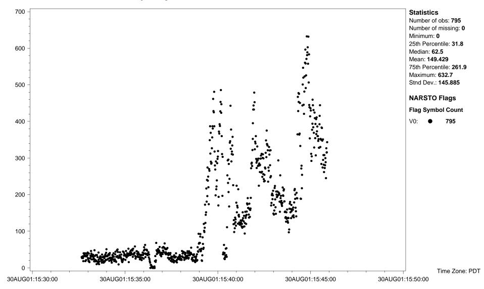
Site ID: **PC01CABCCONV** Variable name: **Particles: count** Units: **number/cm3** Basis: **channel 3** Sampling interval: **1 second** Sampling frequency: **Same as sampling interval** Observation type: **Particles** Particle diameter--lower bound (UM): **0.165** Particle diameter--median (UM): **0.178**
