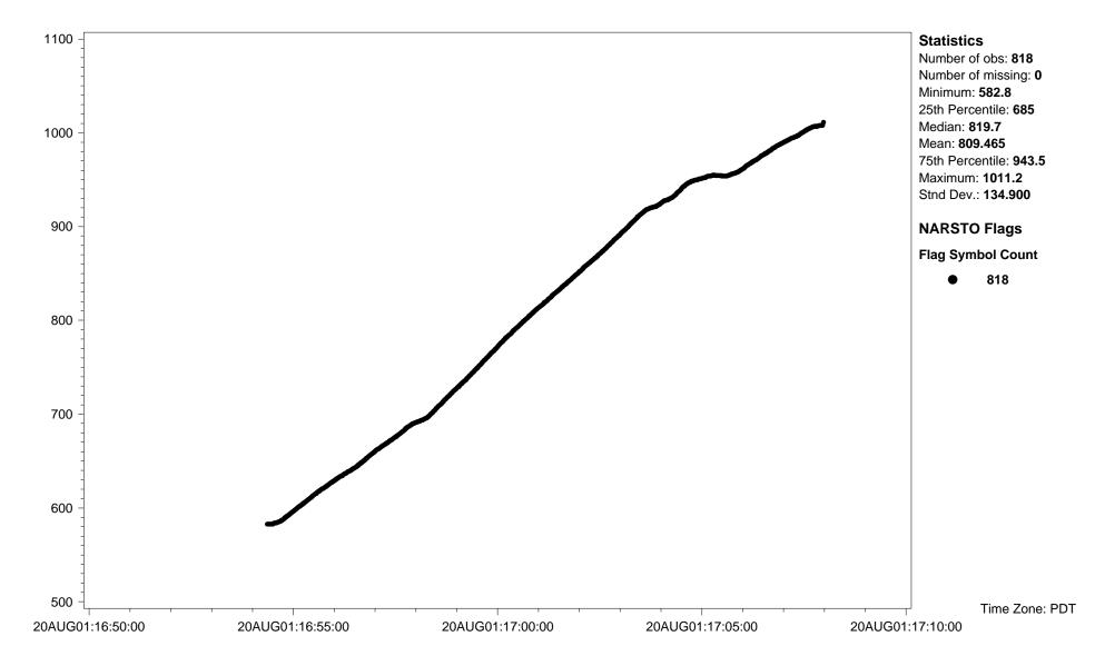
Site ID: PC01CABCCONV Variable name: Temperature: air Units: deg C Sampling interval: 1 second Sampling frequency: Same as sampling interval Observation type: Supplementary data Field sampling or measurement principle: Ultraviolet absorption Sampling Height above ground (m): Varies--see variable Alti Instrument name and model number: Rosemount Static Temperature Measurement principal investigator: Dr. Shao-Meng Li Detection Limit: 2 to 3
