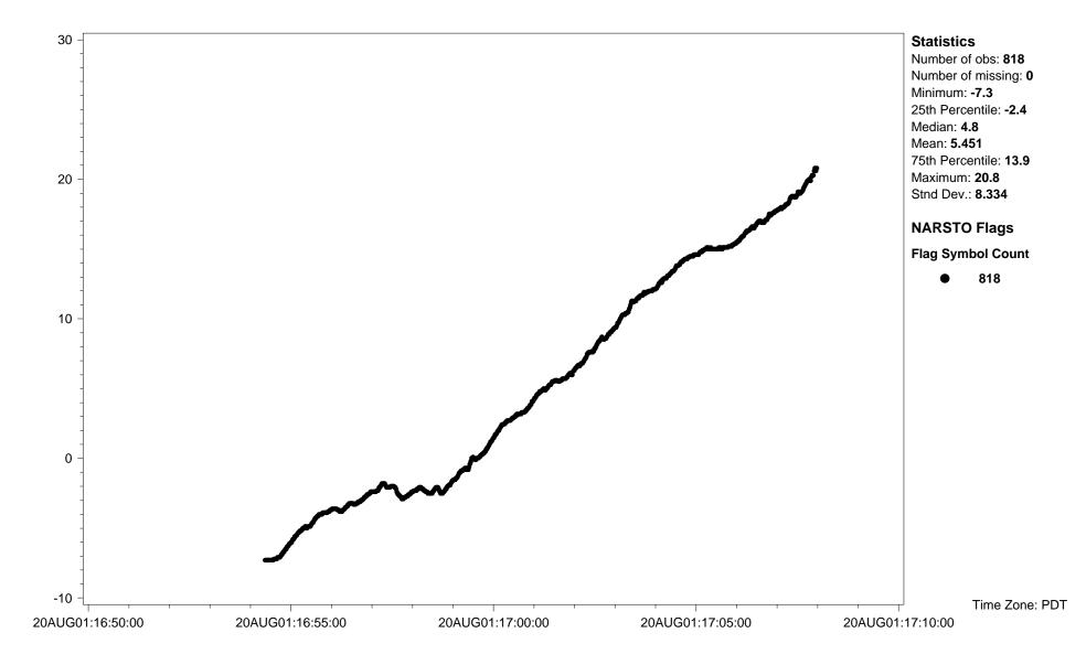
Site ID: PC01CABCCONV Variable name: Temperature: dew point Units: deg C Sampling interval: 1 second Sampling frequency: Same as sampling interval Observation type: Supplementary data Field sampling or measurement principle: Aircraft instrumentation Sampling Height above ground (m): Varies--see variable Alti Instrument name and model number: EG+G Hygrometer Measurement principal investigator: Dr. Shao-Meng Li Detection Limit: Not available
