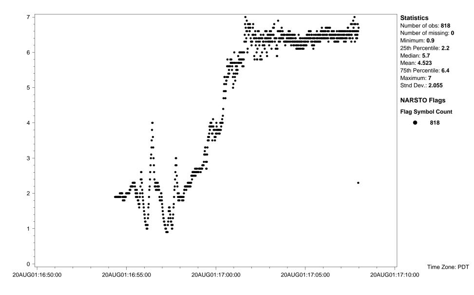
Site ID: PC01CABCCONV Variable name: Ozone Units: ppbv Sampling interval: 1 second Sampling frequency: Same as sampling interval CAS ID: C10028-15-6 Observation type: Gas Field sampling or measurement principle: Ultraviolet absorption Inlet type: Filter in front of sampling line Blank Correction: Not blank corrected Sampling Height above ground (m): Varies--see variable Alti Instrument name and model number: TECO 49 Measurement principal investigator: Dr. Shao-Meng Li Detection Limit: 2 to 3
