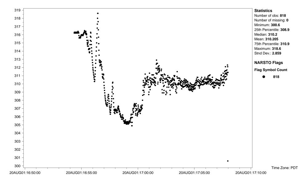
Site ID: PC01CABCCONV Variable name: Temperature: surface Units: deg C Sampling interval: 1 second Sampling frequency: Same as sampling interval Observation type: Supplementary data Field sampling or measurement principle: Radiometer Sampling Height above ground (m): Varies--see variable Alti Instrument name and model number: Barns RadiometerPRT-5 Measurement principal investigator: Dr. Shao-Meng Li
