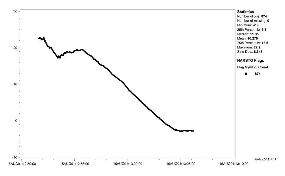
Site ID: PC01CABCCONV Variable name: Temperature: dew point Units: deg C Sampling interval: 1 second
