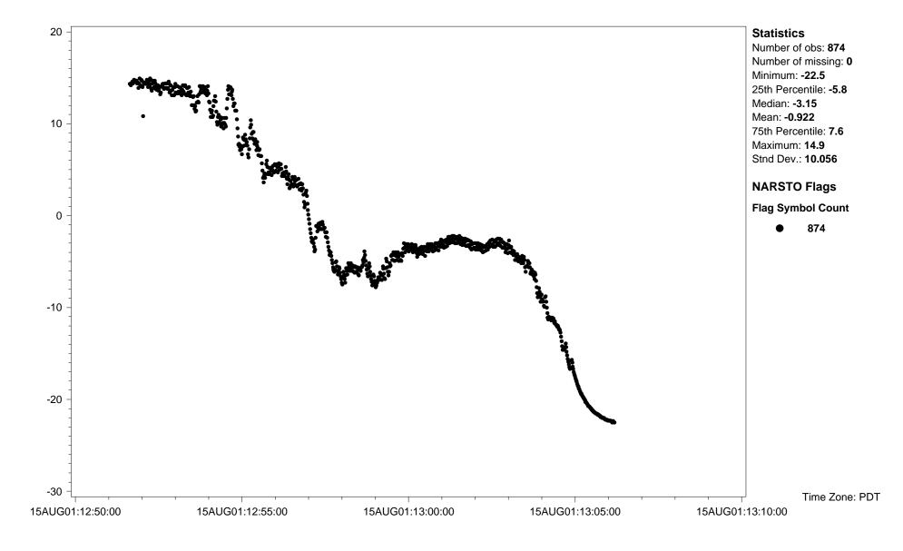
Site ID: PC01CABCCONV Variable name: Temperature: potential equivalent Units: K Sampling interval: 1 second
