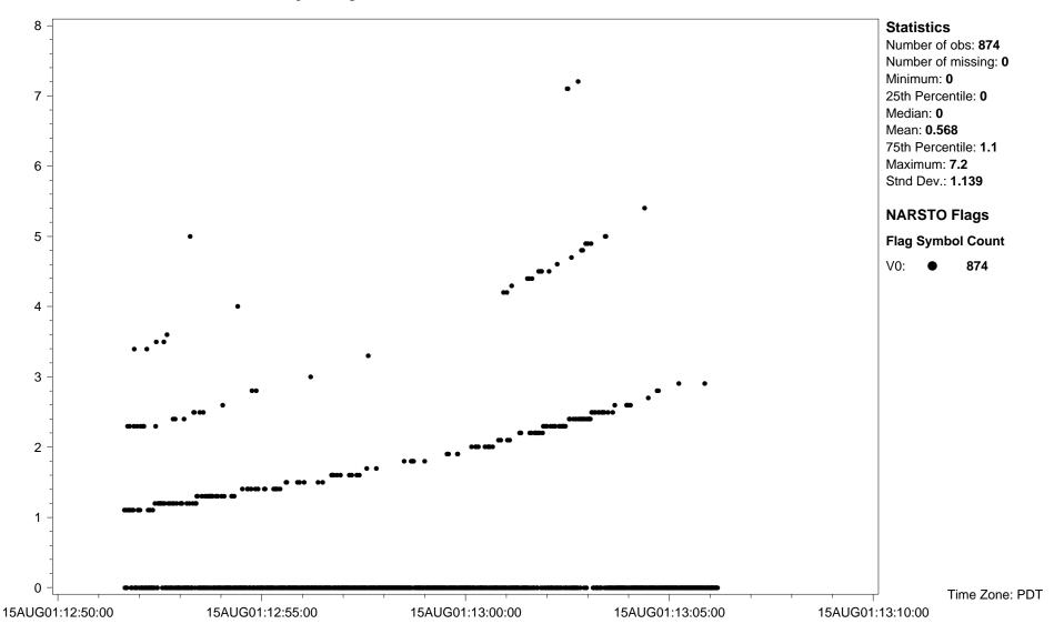
Site ID: PC01CABCCONV Variable name: Particles: count Units: number/cm3 Basis: channel 11 Sampling interval: 1 second Sampling frequency: Same as sampling interval Observation type: Particles Particle diameter--lower bound (UM): 0.930 Particle diameter--upper bound (UM): 1.200 Particle diameter--median (UM): 1.065
