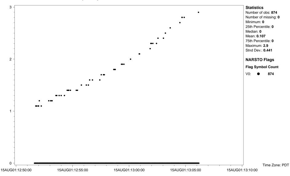
Site ID: PC01CABCCONV Variable name: Particles: count Units: number/cm3 Basis: channel 13 Sampling interval: 1 second Sampling frequency: Same as sampling interval Observation type: Particles Particle diameter--lower bound (UM): 1.500 Particle diameter--upper bound (UM): 2.000 Particle diameter--median (UM): 1.750
