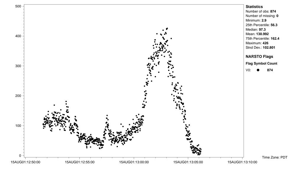
Site ID: PC01CABCCONV Variable name: Particles: count Units: number/cm3 Basis: channel 7 Sampling interval: 1 second Sampling frequency: Same as sampling interval Observation type: Particles Particle diameter--lower bound (UM): 0.340 Particle diameter--upper bound (UM): 0.470 Particle diameter--median (UM): 0.405
