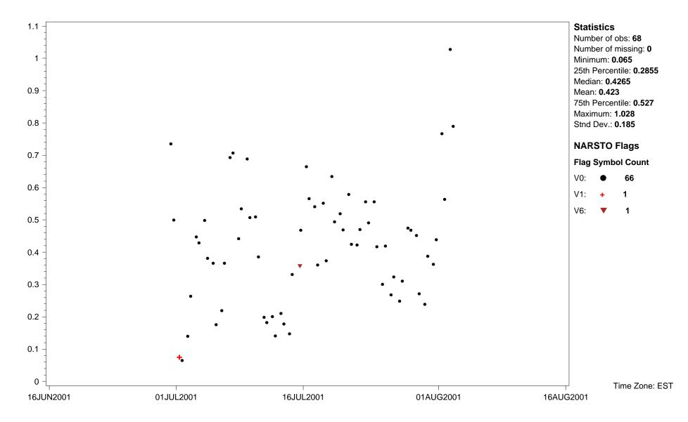
Site ID: **STIFCAONSIM** Variable name: **Sample: total volume** Units: **m3** Sampling interval: **8 h day/16 h night** Sampling frequency: **2 times per day** Observation type: **Flow** Field sampling or measurement principle: **Mass flow controller** Inlet type: **Cyclone** Volume standardization: **25 deg. C; 1 atmosphere** Sampling Height above ground (m): **2** Instrument name and model number: **RAAS2.5-400** Measurement principal investigator: **Jeffrey Brook**
