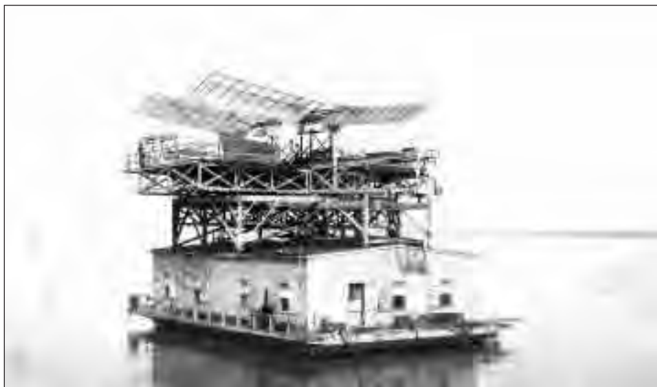
What the public acknowledged about powered flight after December 1903 was the ignominious, highly publicized failure of Samuel P. Langley's Great Aerodrome , not the successful flights of the Wrights, which few knew about and even fewer believed had actually happened. Here, Langley's Great Aerodrome rests on its catapult atop a houseboat, ready for flight, on 8 December 1903. SI Negative No. A-18789
