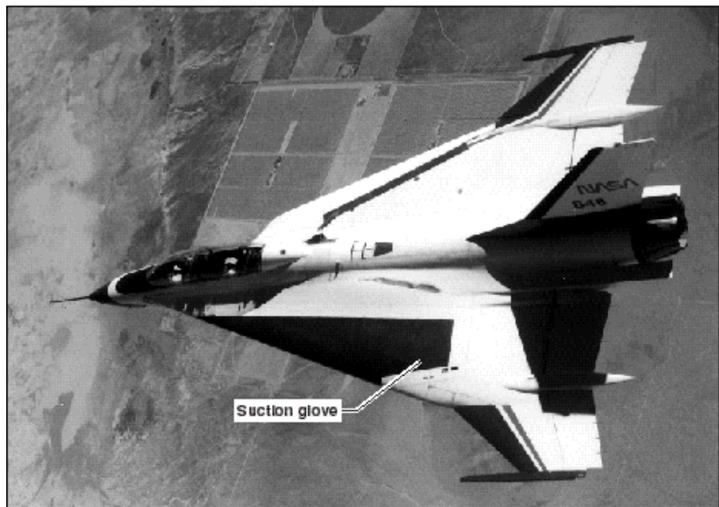
Figure 19. Two-seat F-16XL Supersonic Laminar-Flow-Control flight research aircraft with a suction glove installed on the left wing. (NASA photo EC96-43831-5 by Jim Ross).
