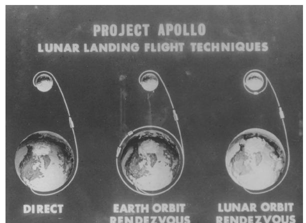
A diagram from 1962 demonstrating the three basic approaches considered for lunar landing missions.
