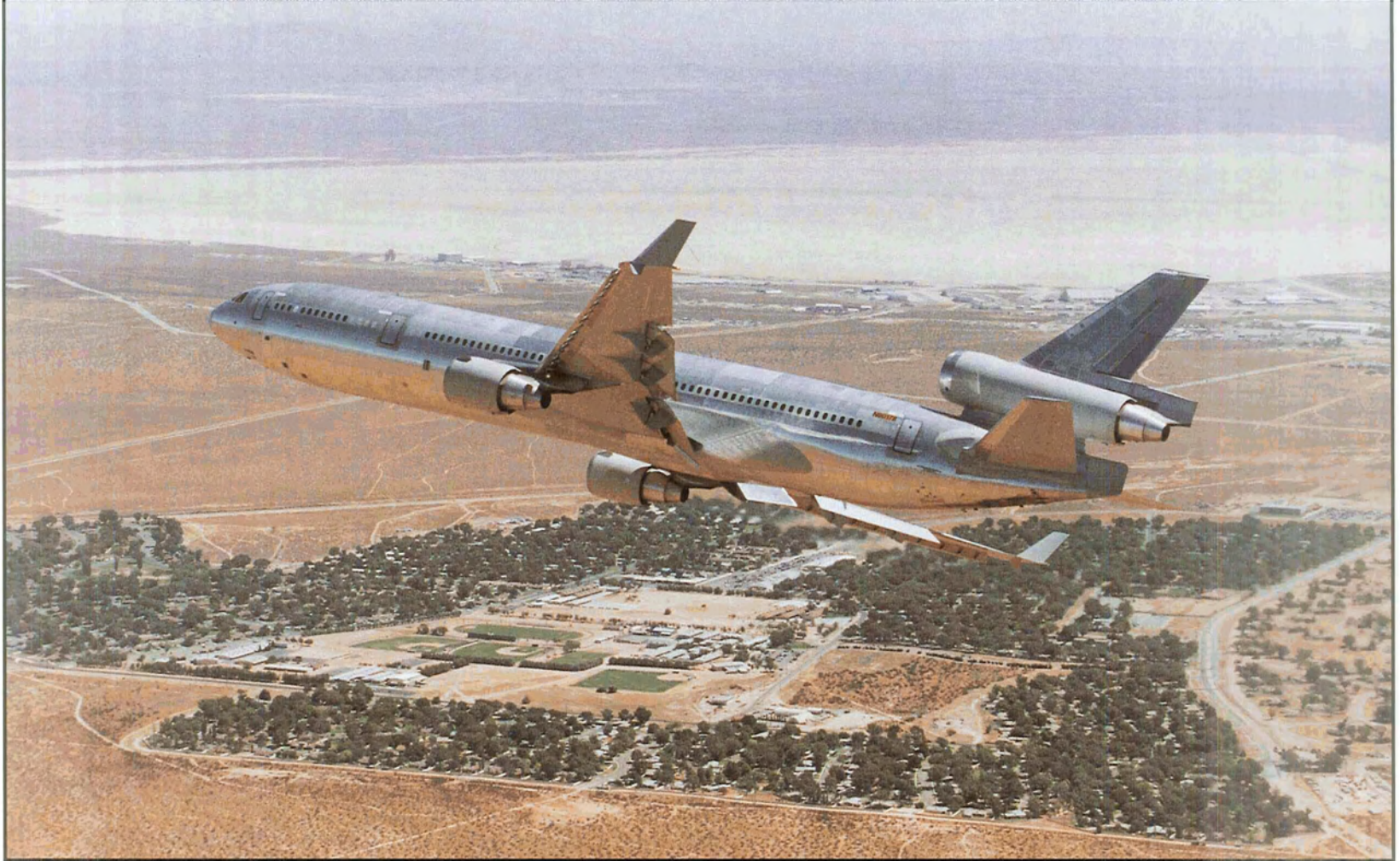
MD-11 showing one application of the winglet concept in a production aircraft. Winglets produce a forward force component (thrust) in the vortices that usually swirl off of conventional wingtips, thereby reducing the overall drag of the airplane. Developed by Richard Whitcomb at Langley Research Center, winglets demonstrated in flight research at Dryden in 1979 and 1980 that they could increase an aircraft's range by up to seven percent at cruise speeds. (NASA Photo EC95 43247-5)
