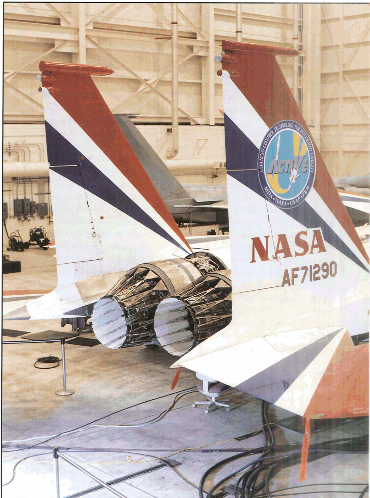
F-15 Advanced Control Technology for Integrated Vehicles (ACTIVE) aircraft showing the thrust-vectoring nozzles that promised to improve aircraft efficiency and control (NASA Photo EC95 43273-4)
