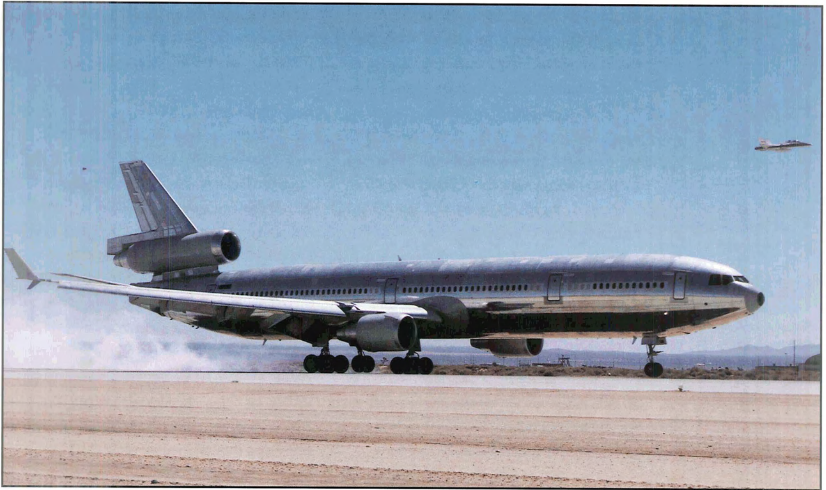
MD-11 Propulsion Controlled Aircraft (PCA) about to touch down in the milestone first throttles-only landing of a transport aircraft on 29 August 1995, with F/A-18 chase aircraft in the background (NASA Photo EC95 43247-4)
