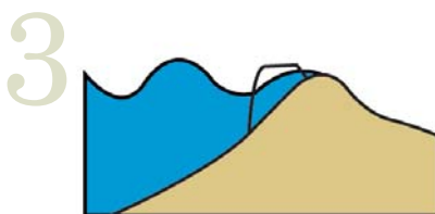
Impact Level 3: Waves overtop the barrier island. If waves reach over the dune, or if there is no dune, sand will be pushed landward. Over time, the island will migrate toward land.
