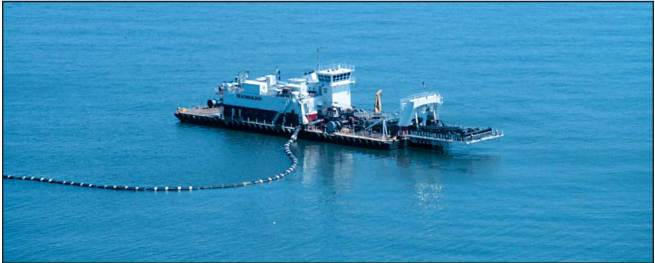
A dustpan dredge, the “Beach Builder”, used in the restoration of East Timbalier Island.
