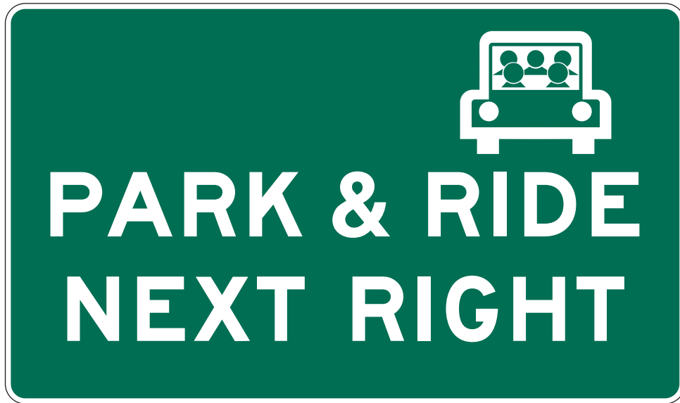
Figure 2E-18. Supplemental Guide Sign for a Park and Ride Facility (Route without Exit Numbering)
