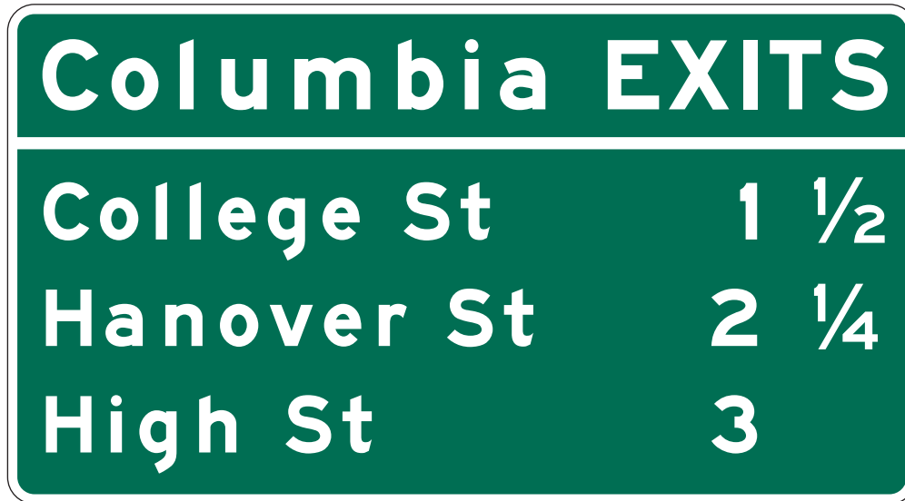
Figure 2E-26. Community Interchanges Identification Sign
