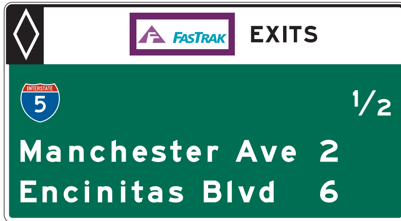
Figure 2E-49. Example of an Exit Destinations Sign for an HOV/Toll Managed Lane
