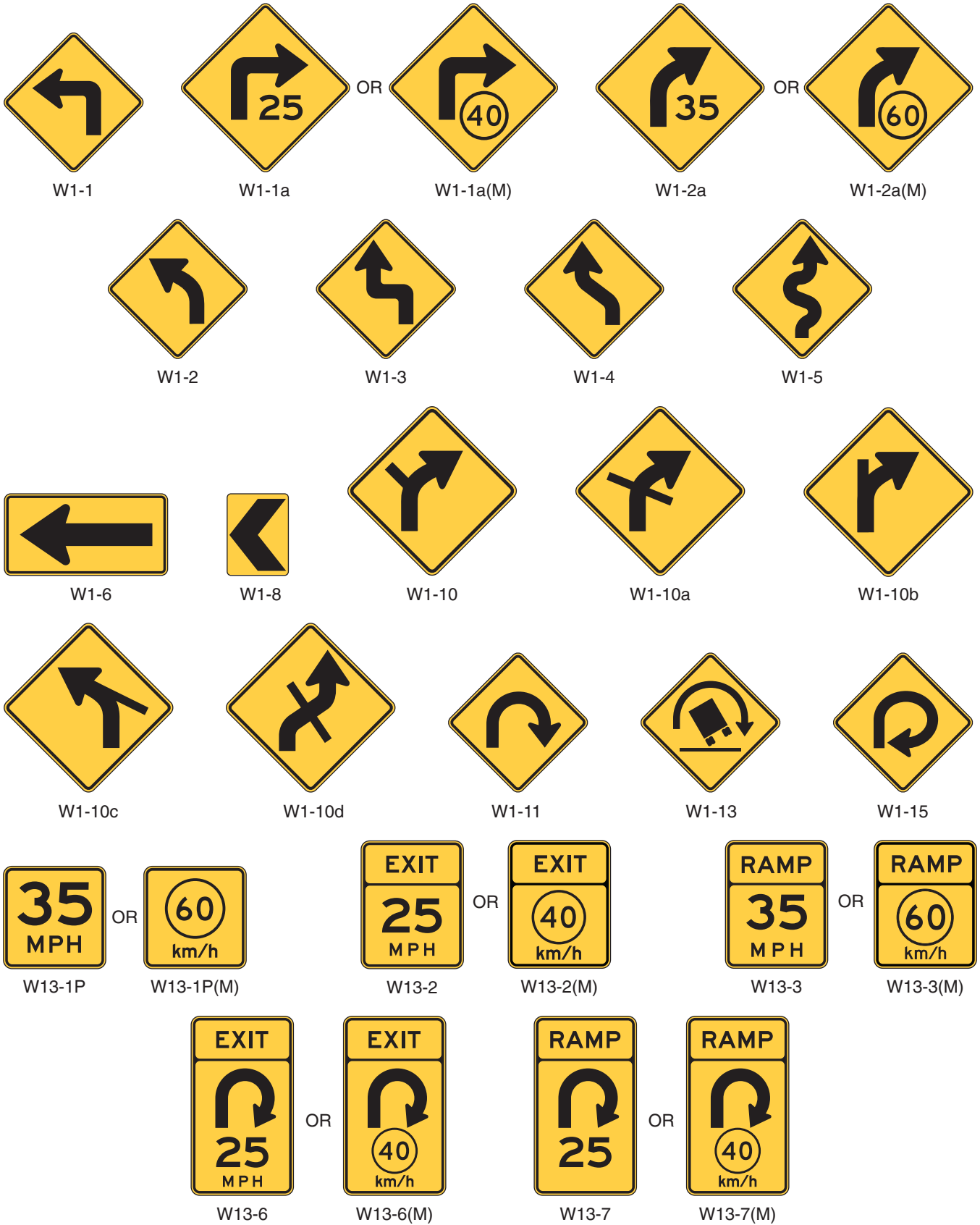
Figure 2C-1. Horizontal Alignment Signs and Plaques
