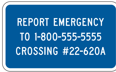
Figure 10C-5. Example of Emergency Notification Sign
