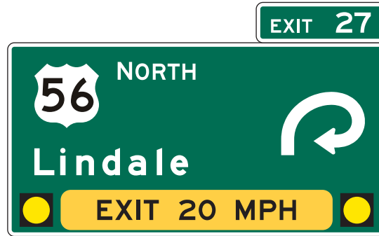
Exit Direction sign with E13-2 sign panel and flashing yellow beacons
