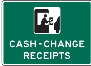
Attended Lane with Required M4-17 Toll Collector Symbol
