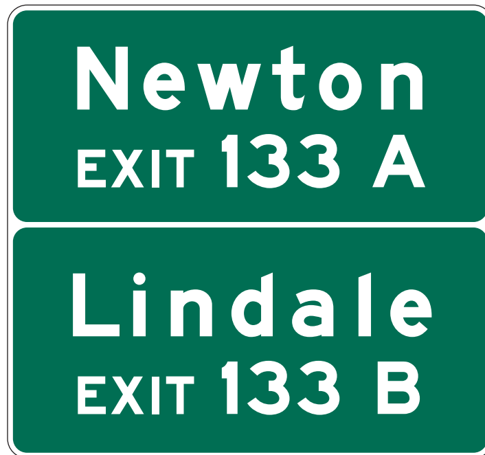
Figure 2E-17. Supplemental Guide Signs for Multi-Exit Interchanges
