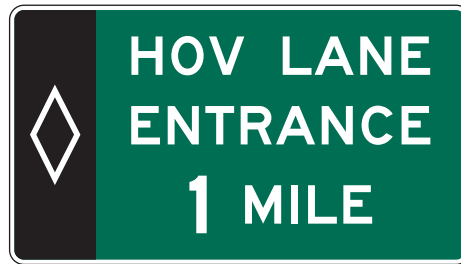
Figure 2E-46. Example of an Overhead Advance Guide Sign for a Preferential Lane Entrance
