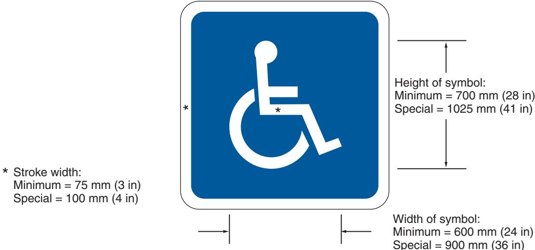
Figure 3B-22. International Symbol of Accessibility Parking Space Marking with Blue Background and White Border Options
