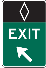
Figure 2E-47. Exit Gore Sign for a Direct Exit from a Preferential Lane
