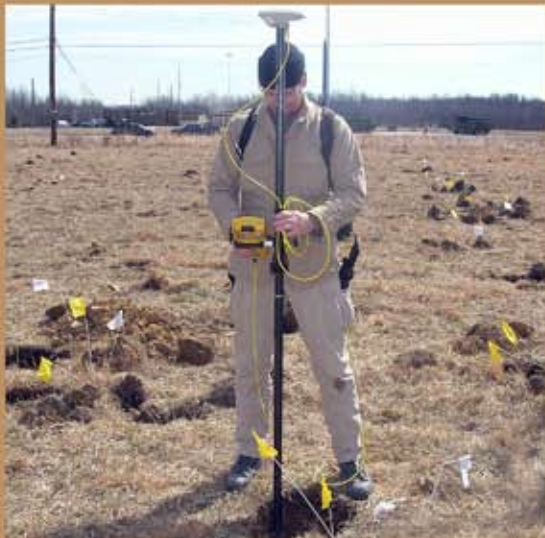
The GPS system is being used to measure the location of an anomaly.
