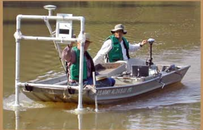
Demonstrator displaying their shallow water detection system.
