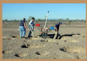
The EM61 in the pushcart platform is shown being demonstrated by Shaw Environmental, Inc. at Yuma Proving Ground, Arizona.
