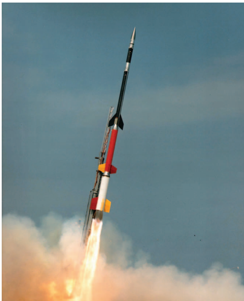
FIGURE 7.1 A Black Brant XII sounding rocket carrying aloft an experiment to measure atomic oxygen emissions in Earth's upper atmosphere. Sounding rockets are used for a variety of important research objectives in solar and space physics, from in situ study of ion acceleration processes in the high-latitude ionosphere to remote-sensing observations of the Sun's corona. Because they are relatively inexpensive and require less time to develop and implement than satellite investigations, sounding rocket experiments have proven to be a valuable education asset for training as well as an important research tool. Courtesy of P.J. Eberspecker (NASA Wallops Flight Facility).
