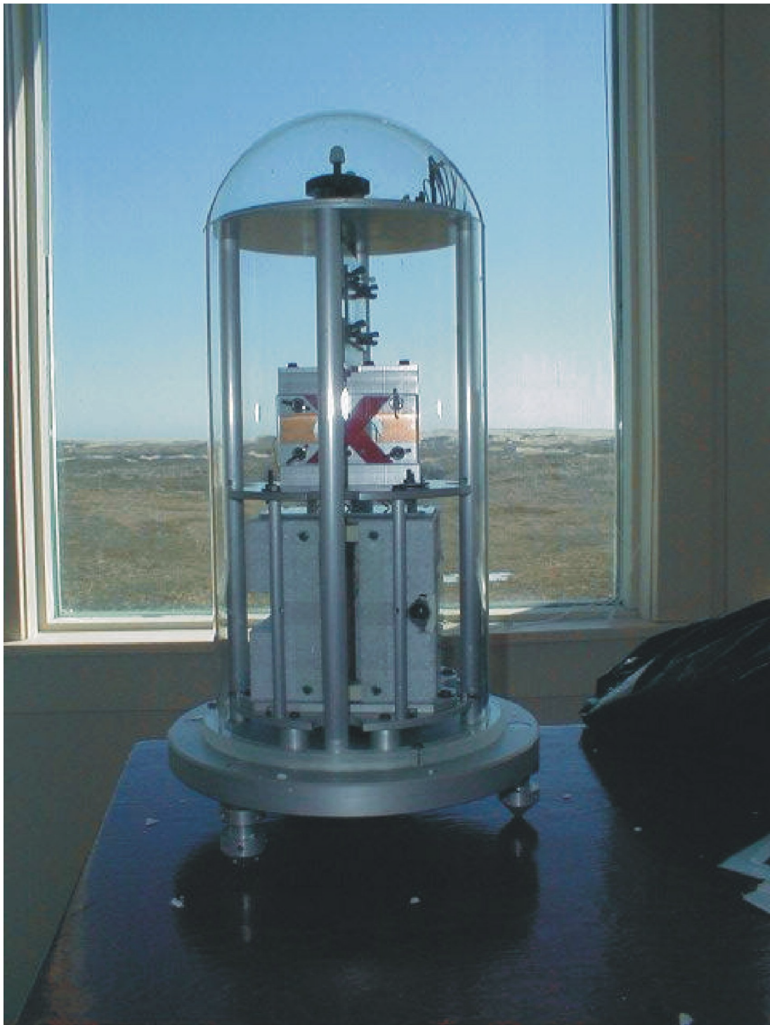
Danish Meteorological Institute triaxial fluxgate magnetometer
