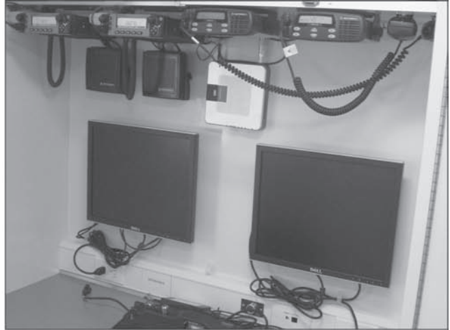
Interior of the Jackson Police communications vehicle, showing a work desk with two computer monitors and wireless Internet
