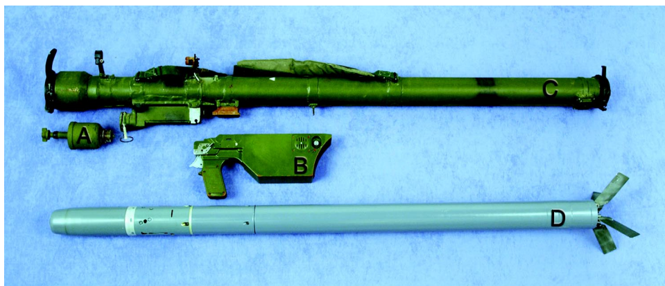
Figure 1: Components of a Man-Portable Air Defense System
